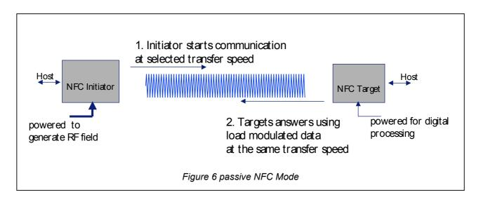
The PN531's firmware and contactless UART handle the NFC protocol.
