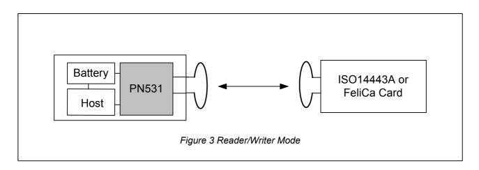
In the reader/ writer mode the PN531 enables communication to a passive ISO14443A/MIFARE<sup>®</sup> or FeliCa<sup>™</sup> card.
