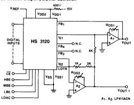
Connection Diagram, Bipolar Operation (for applications where bipolar offset temperature drift (≈ 10 ppm/°C) is not critical)
