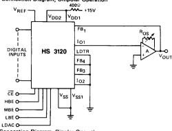
Connection Diagram, Bipolar Operation
