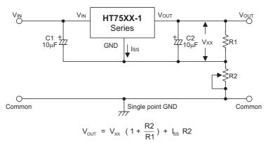
**Circuit for Increasing Output Voltage**
