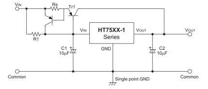
**Circuit for Increasing Output Voltage**
