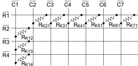
All the resistors are 330k $\Omega$ . The resistor option functions and the default specifications (without option resistors) are listed below (HT9320A/B/C/K/L).
