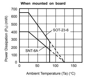
Figure 11 Power Dissipation of Package
