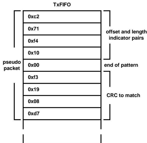
Table 2-1 deciphers the pseudo packet in Figure 2-2 indicating the relative offset and length indicators which the IP1000A LF will apply to all receive frames.
