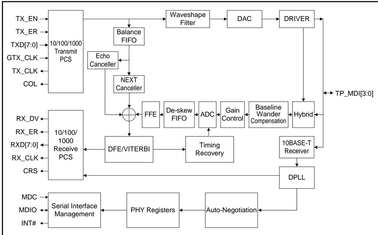
With state-of-the-art DSP mixed-mode technology, the physical layer of IP1000A LF is designed to accomplish low power, high performance, and full integration for 1000BASE-T, 100BASE-TX, and 10BASE-T operation.
