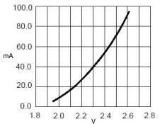
Forward Current vs. Forward Voltage
