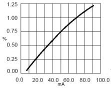
Relative Luminous Flux vs. Forward Current
