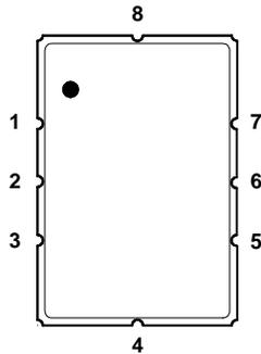
\*Enable Sense: Pin 2 Ground-Clock Off
