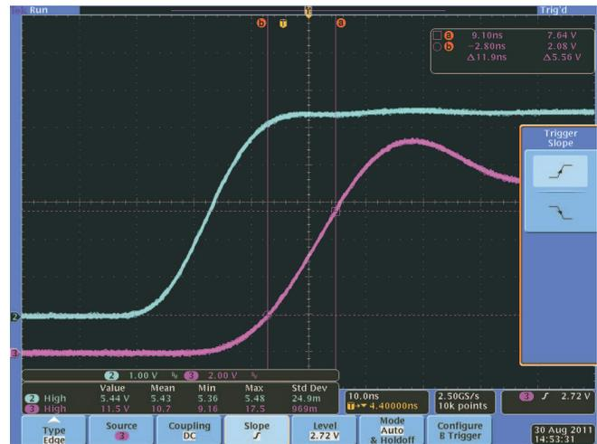
Figure 26. Typical Turn-Off Waveform (VDD = 10 V, C<sub>L</sub> = 1 nF)
