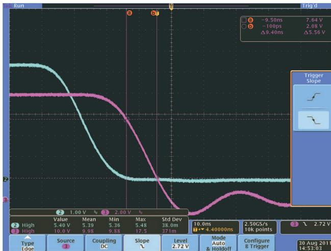
Figure 25. Typical Turn-On Waveform (VDD = 10 V, C<sub>L</sub> = 1 nF)
