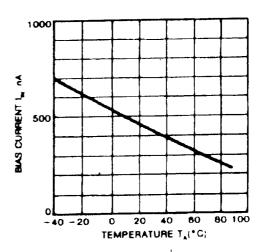
DIFFERENTIAL AMPLIFIER OUTPUT CURRENT-TEMP
