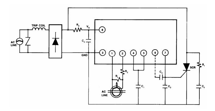
Supply voltage circuit is connected as a previous diagram. Please decide constants R1, R2, C4, and C5 of a filter in order to keep at least 12V in Vs, when normal supply current flows.
