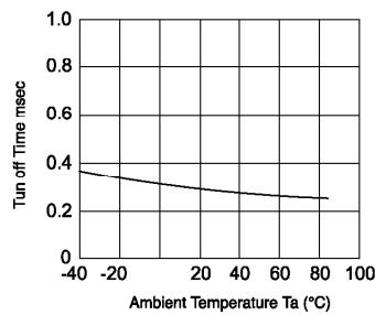
**Fig.5** LED operate vs. ambient temperature
