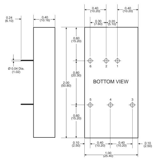
$\begin{array}{lll} \text{ALL DIMENSIONS IN INCHES (mm)} \\ \text{Tolerance} & : \pm 0.008 \; (0.2) \; \text{max. on pin placement} \\ & \pm 0.02 \; (0.5) \; \text{max. on outer dimensions} \end{array}$
