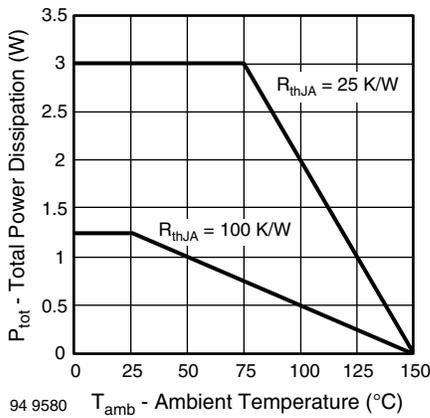
Fig. 2 - Typ. Total Power Dissipation vs. Ambient Temperature
