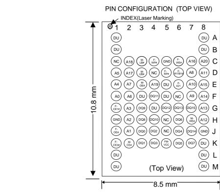
FM-VCC : VCC for Flash / Mobile RAM F-RP# : Reset power down for Flash
