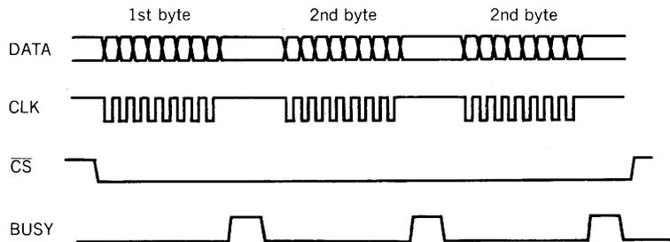
The internal data processing is performed on input of every one byte (8 bits).
