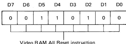
When this command is executed, Display OFF, Locsc Oscillation ON, and Video RAM Write mode are automatically set and these settings remain unchanged until execution of other commands even after the Video RAM All Reset command.
