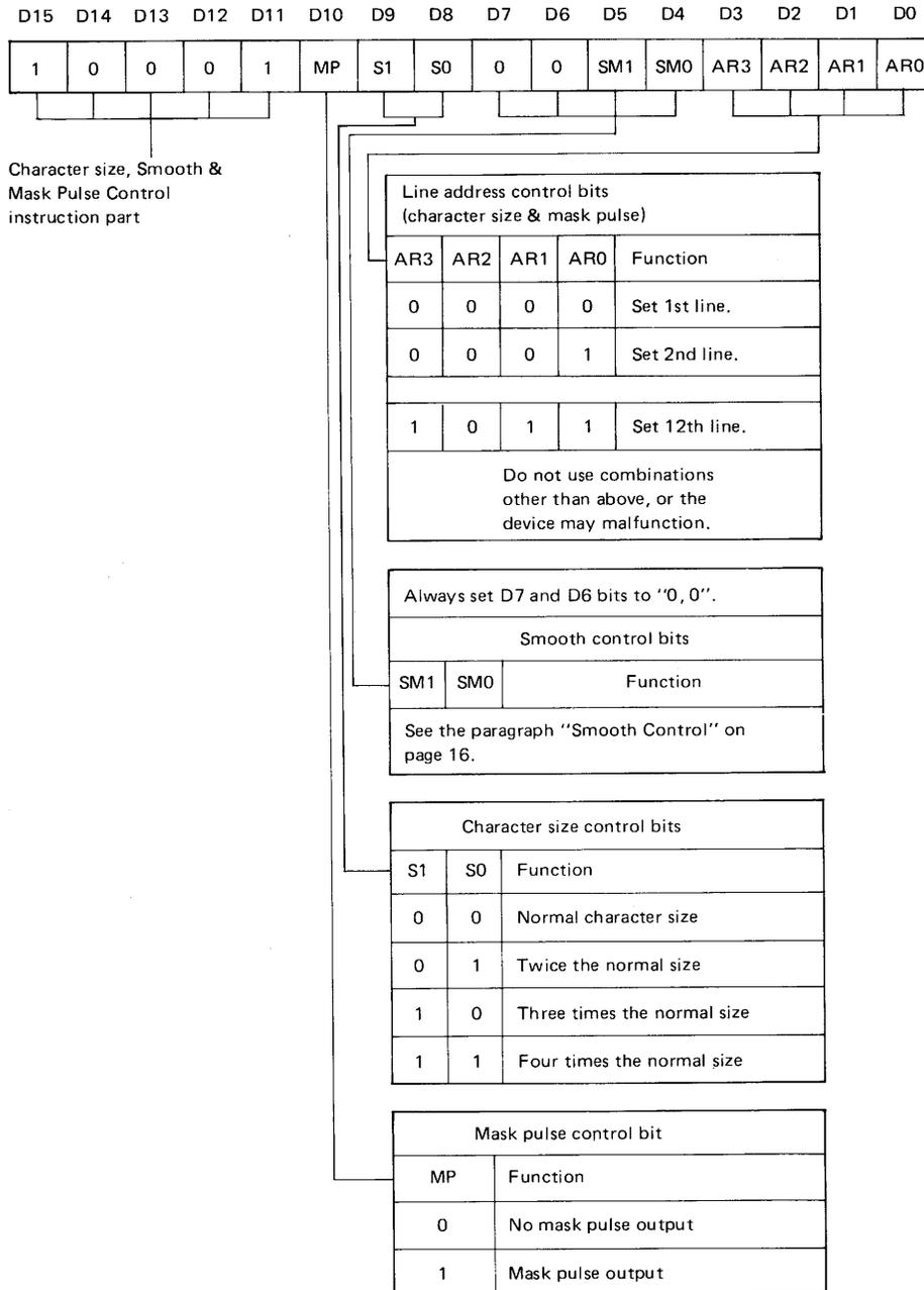
**Note:** The MP (mask pulse) control bit is valid only when the mask pulse function has been selected with the Mask code option. If this function has not been selected, set the MP bit to "0".
