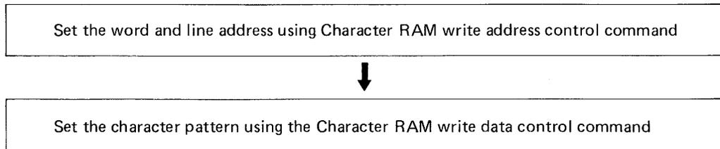
Both the CRAM word address and line address are incremented by the STB signal as shown below. Therefore, this address may be set only once to write 16 characters continuously.
