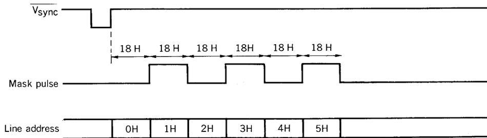
The leading and trailing edges of the mask pulse are synchronized with the trailing edge of  $\overline{H_{SYNC}}$ .
