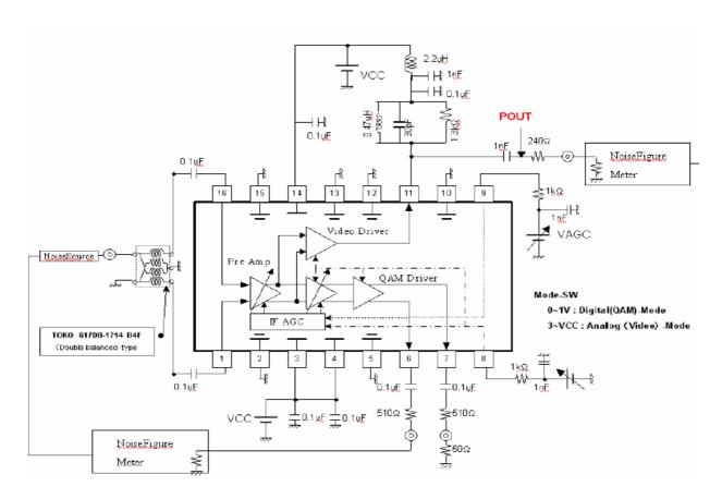
Note Balun Transformer: TOKO 617DB-1714 B4F (Double balanced type)
