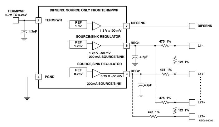
Figure 1. Low-Voltage Differential Discrete Resistor Stack
