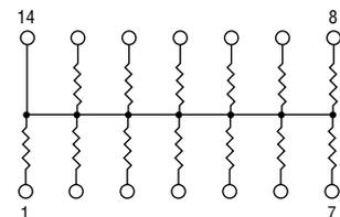
These models incorporate 7, 13, 15, 17, or 19 thin-film resistors of equal value, each connected by a common pin.
