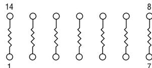
These models incorporate 4, 7, 8, 9, or 10 thin-film resistors of equal value, each connected between a separate pin.
