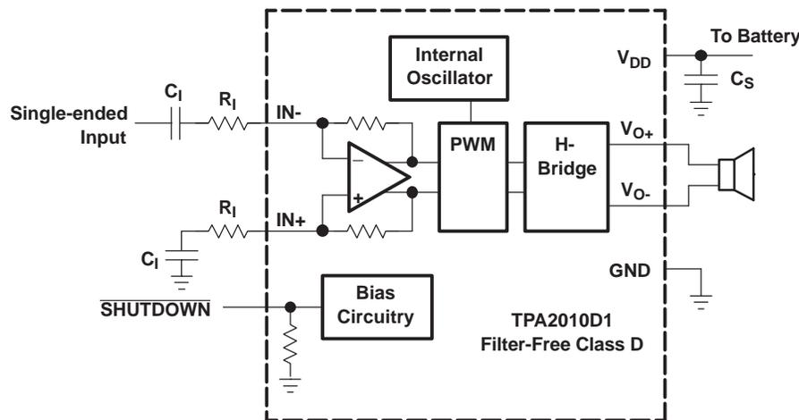
Figure 29. TPA2010D1 Application Schematic With Single-Ended Input
