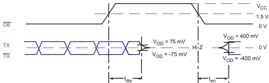
Figure 6. TMDS Enable and Disable Timing Definitions
