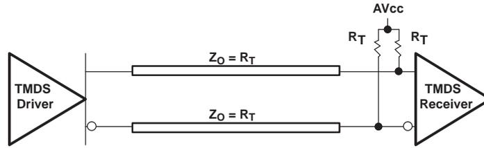
Figure 1. Typical Termination for TMDS Output Driver
