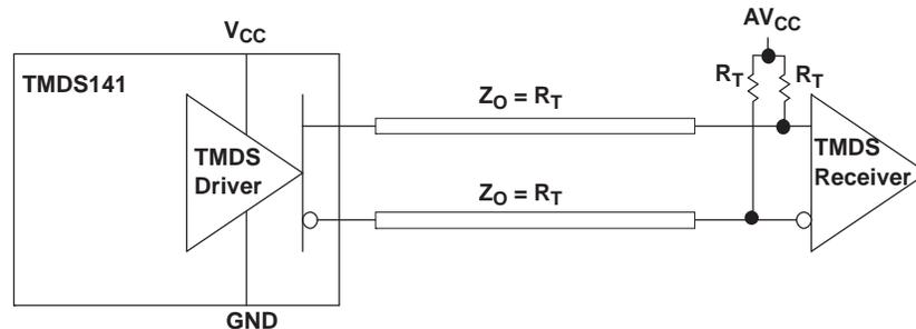
Figure 17. TMDS Driver and Termination Circuit
