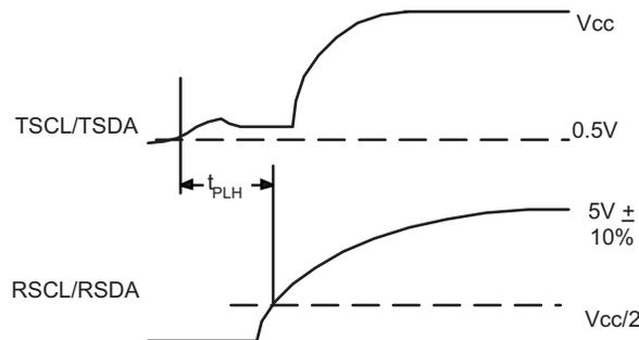
**Figure 19. Waveform of Turning Driver T Off**
