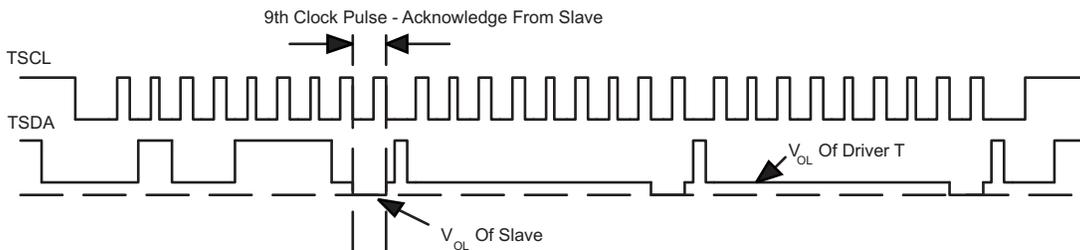
Figure 22. Bus T Waveform
