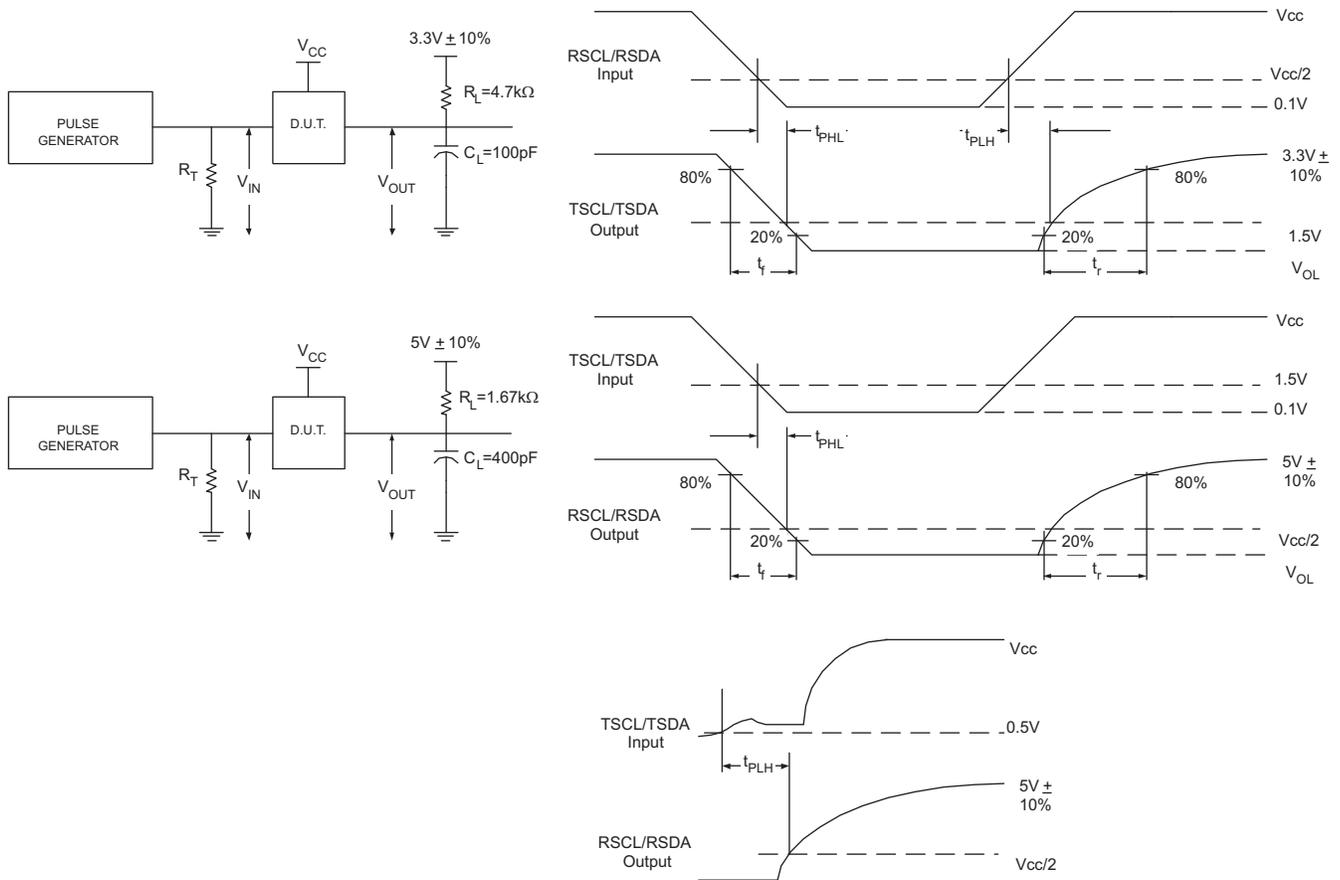
Figure 8. I<sup>2</sup>C Timing Test Circuit and Definition
