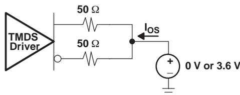
Figure 4. Short Circuit Output Current Test Circuit
