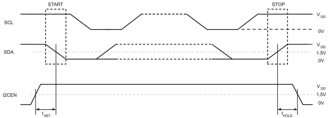
**Figure 9. I<sup>2</sup>C Setup and Hold Definition**
