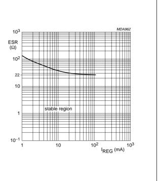
Fig.6 ESR as a function of I<sub>REG</sub> for selecting the value of the output capacitor.
