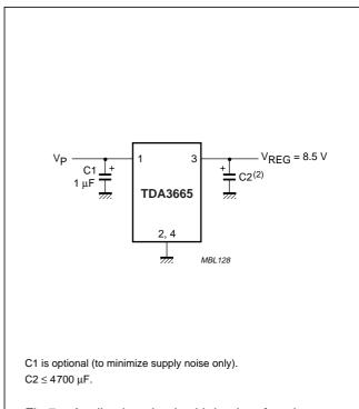
Fig.7 Application circuit with backup function (SO4 version).
