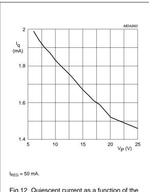
Fig.12 Quiescent current as a function of the supply voltage.
