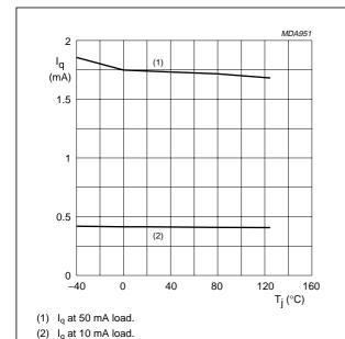
Fig.10 Quiescent current as a function of the junction temperature.
