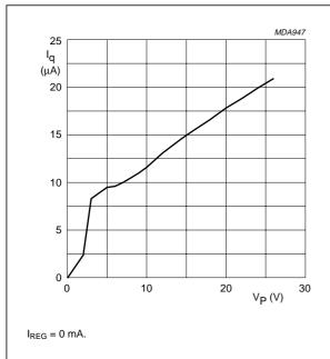
Fig.8 Quiescent current as a function of the supply voltage.
