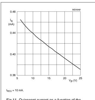
Fig.11 Quiescent current as a function of the supply voltage.
