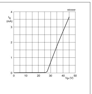
Fig.9 Quiescent current increase as a function of high supply voltage.
