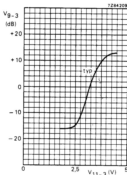
Fig. 6 Treble control curve;  $f = 15 \text{ kHz}$ ;
