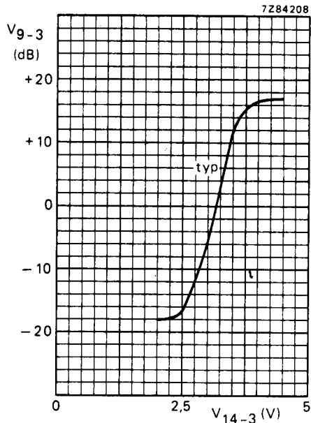
Fig. 5 Bass control curve;  $f = 40 \text{ Hz}$ ;
