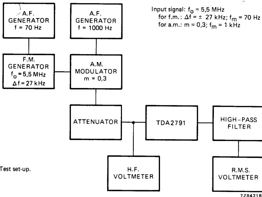
Fig. 4 Test set-up.
