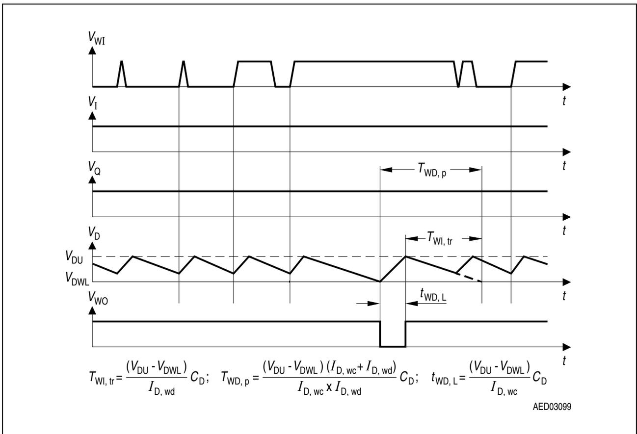
**Figure 8** Timing of the Watchdog Function
