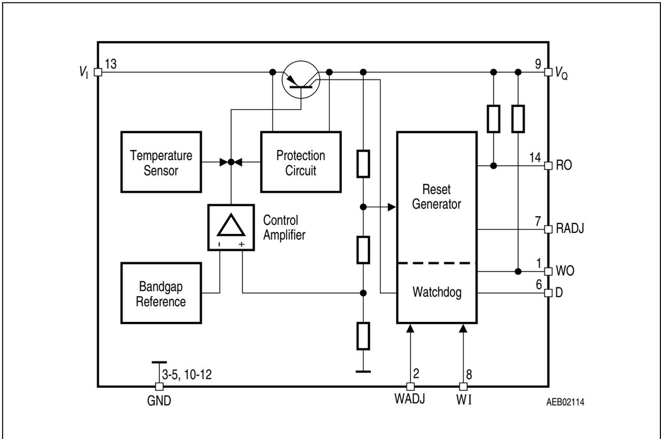
**Figure 2** Block Diagram
