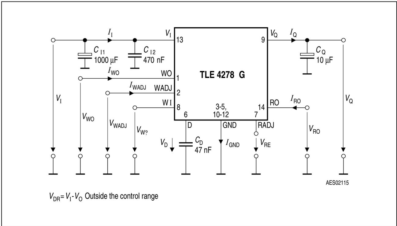
**Figure 3 Test Circuit**
