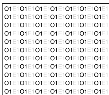
Figure 9. Odd Pixels from Frame 1
