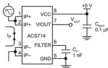
Application 1. The ACS714 outputs an analog signal,  $V_{OUT}$ , that varies linearly with the uni- or bi-directional AC or DC primary sensed current,  $I_P$ , within the range specified.  $C_F$  is recommended for noise management, with values that depend on the application.
