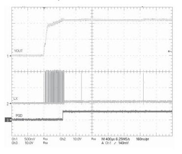
Startup 1.15V 19VBAT 20A load 1 ani YOUT 1111 LX 2 PGD 2.4 Ch1 Ch3 500mV 10.0V B<sub>W</sub> B<sub>W</sub> Ch2 10.0Y BW M 400µs 6.25MS/s A Ch1 ∠ 140mY 160ns/pt
