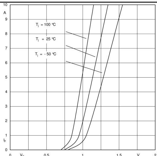
Fig. 1, Forward characteristics (typical values)
