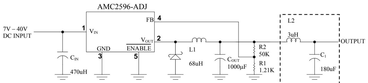
**Figure 3. LC Filter for Low Output Ripple**
