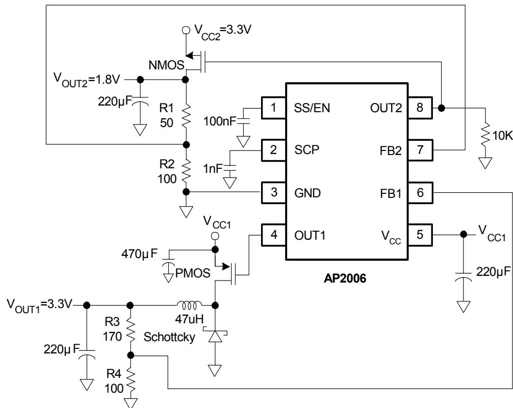
$$\text{AP2006} \Rightarrow V_{\text{OUT1}} = 1.25 * (1 + R3/R4)$$
