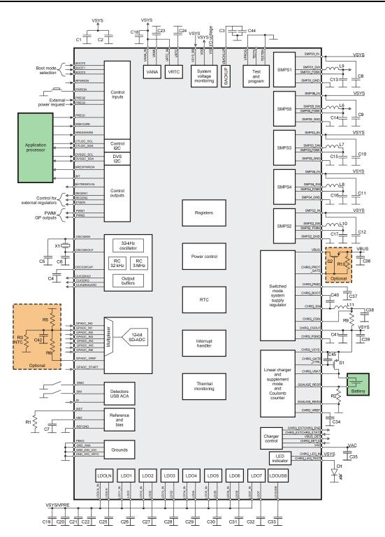
Figure 1. TWL6032 Device Block Diagram
