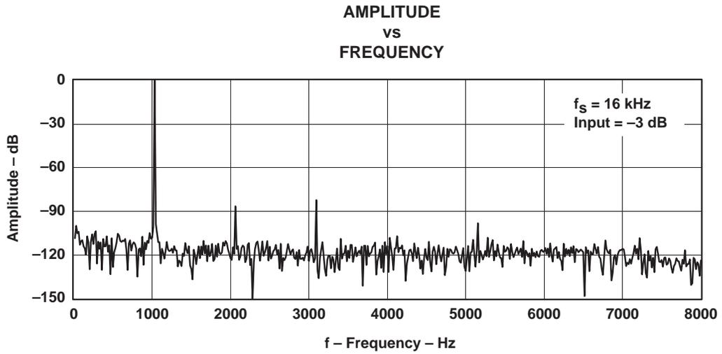
Figure 5-6. FFT-DAC Channel,  $f_s = 16 \text{ kHz}$ , Input = -3 dB
