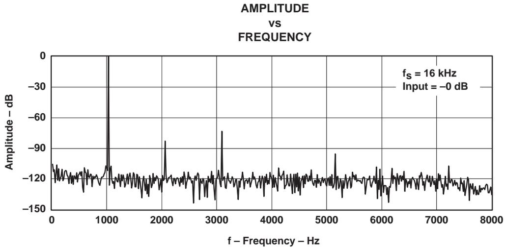
Figure 5-10. FFT-DAC Channel,  $f_s = 16 \text{ kHz}$ , Input = 0 dB
