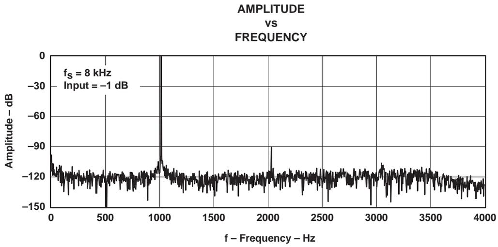
Figure 5-7. FFT-ADC Channel,  $f_s = 8 \text{ kHz}$ , Input = -1 dB
