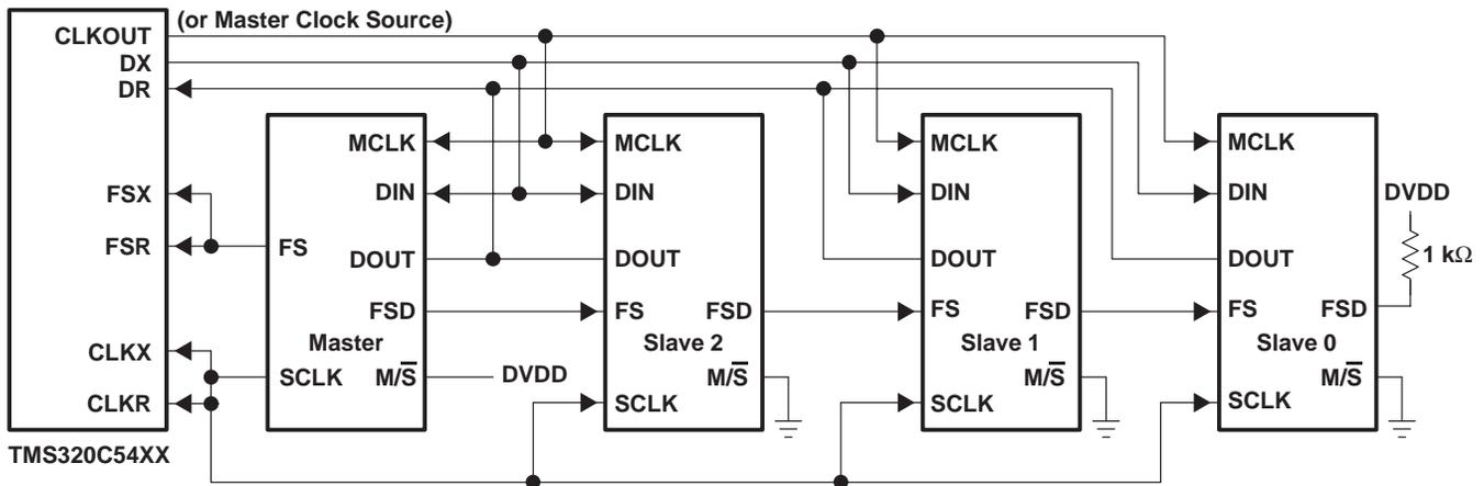
Figure 2–15. Cascade Mode Connection (to DSP Interface)
