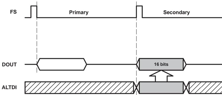
NOTE A: When DIN performs a write operation (sets D12 to 0) during secondary communication.
