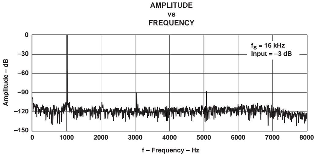
Figure 5-4. FFT-ADC Channel,  $f_s = 16 \text{ kHz}$ , Input = -3 dB
