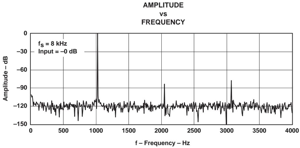
Figure 5-9. FFT-DAC Channel,  $f_s = 8 \text{ kHz}$ , Input = 0 dB
