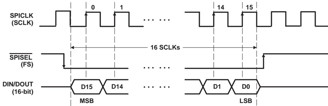
Figure 2–11. Timing Diagram for the SPI\_CP1 Mode (M1M0 = 10)
