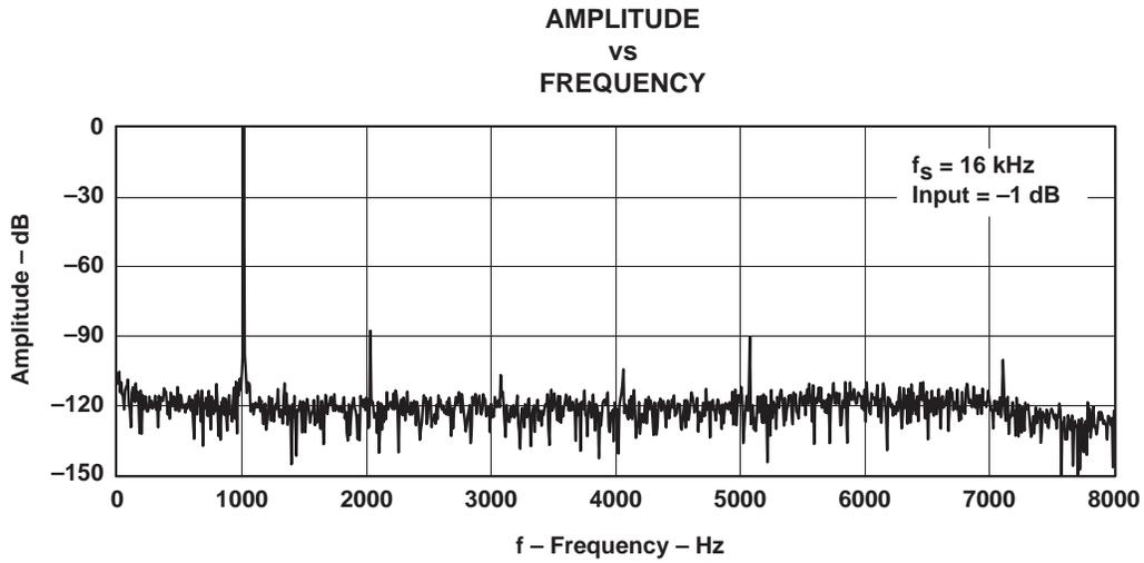
Figure 5-8. FFT-ADC Channel,  $f_s = 16 \text{ kHz}$ , Input = -1 dB
