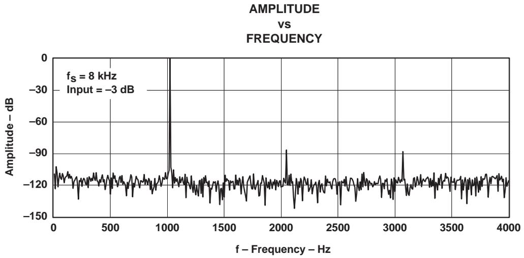
Figure 5-5. FFT-DAC Channel,  $f_s = 8 \text{ kHz}$ , Input = -3 dB
