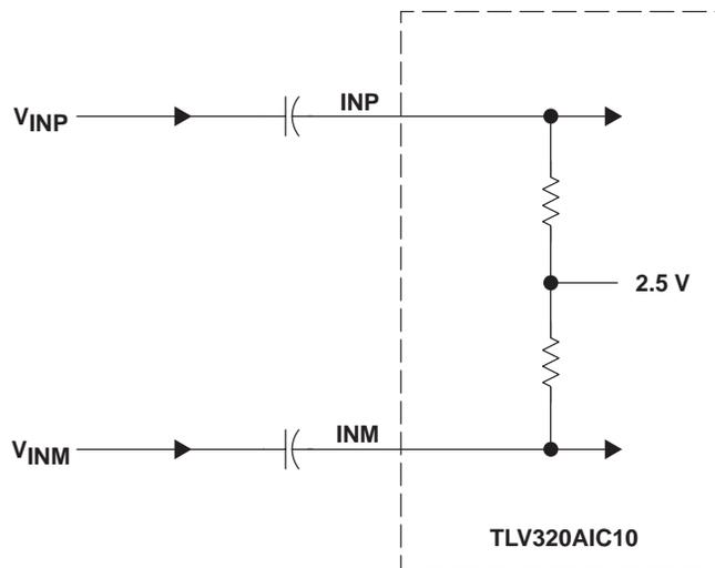
Figure 2–17. INP and INM Internal Self-Biased (2.5-V) Circuit
