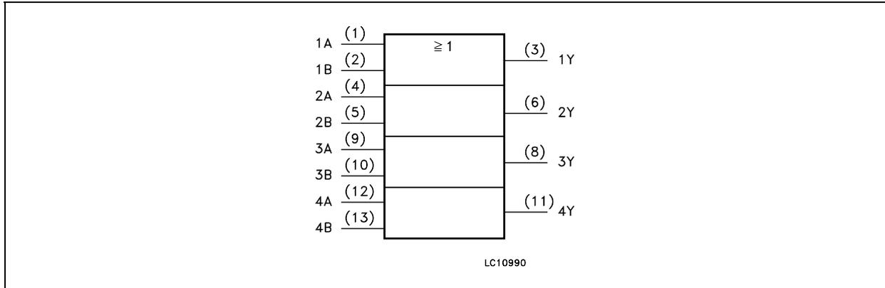
INPUT AND OUTPUT EQUIVALENT CIRCUIT
