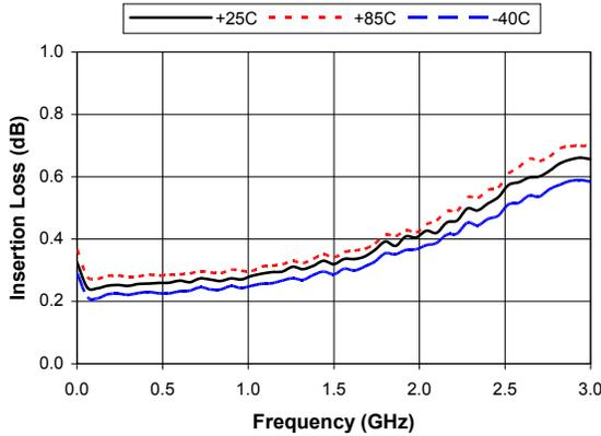
*Insertion Loss with Positive Control*
