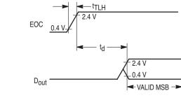
NOTE:  $D_{out}$  is driven only when  $\overline{CS}$  is active (low).
