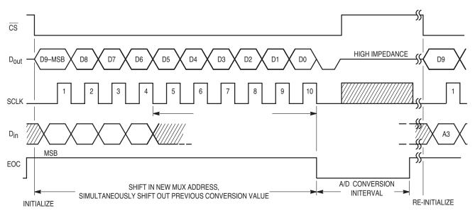
Figure 9. Timing for 10-Clock Transfer Using CS
