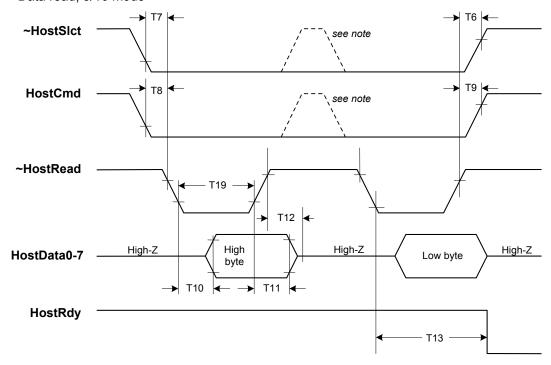
Note: If setup and hold times are met,  $\sim$ HostSlct and HostCmd may be de-asserted at this point.
