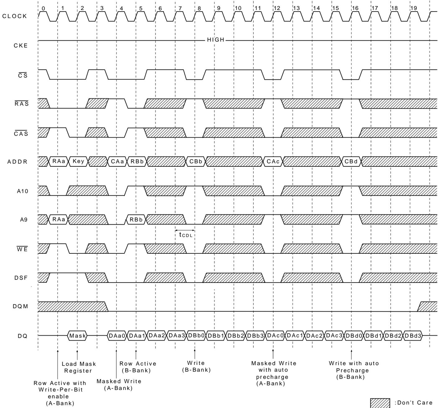
**Read & Write Cycle at Different Bank @ Burst Length =4**
