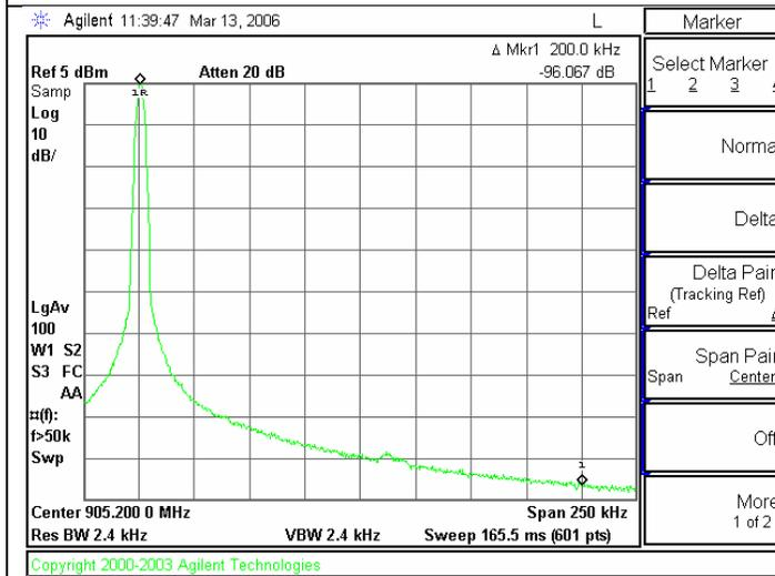
Spur at 200 kHz offset for a frequency of 905.1 MHz is better than -96.0 dBc.
