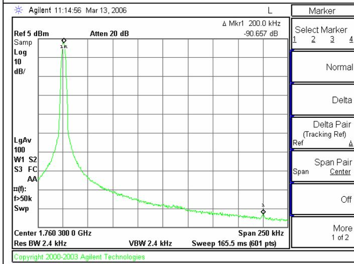
Spur at 200 kHz offset at a worst case frequency of 1760.2 MHz is -90.6 dBc. Worst case channels occur at exactly one channel spacing above or below a multiple of the crystal frequency.
