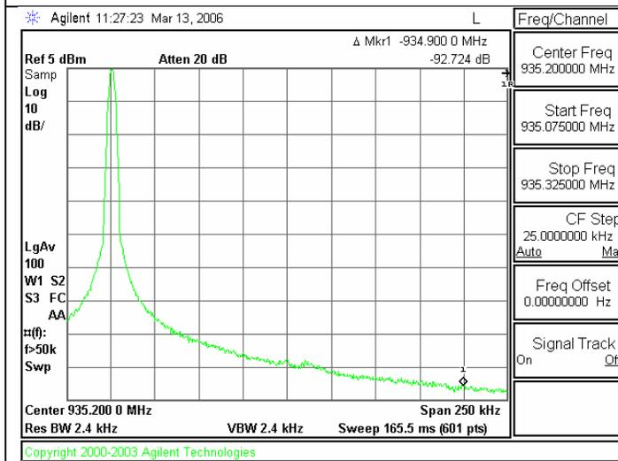
Spur at 200 kHz offset for a frequency of 935.1 MHz is better than -92.7 dBc.
