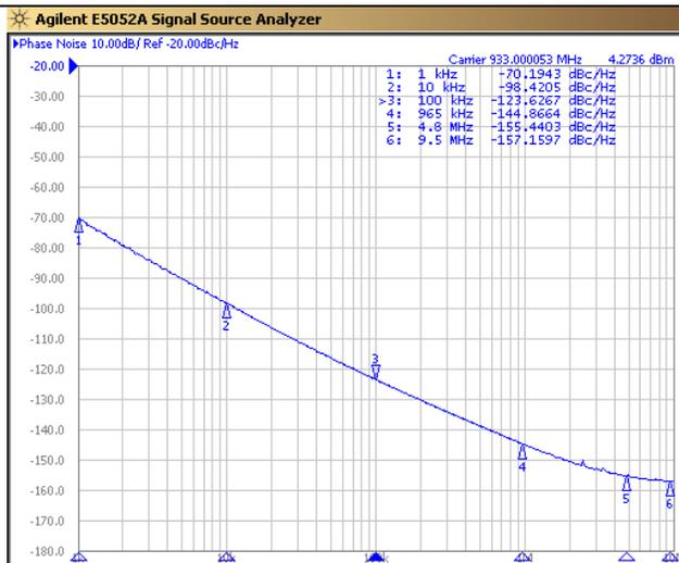
The plots to the left show the true phase noise capability of the VCO. In order to take these plots, a 20 Hz loop bandwidth was used with the E5052 spectrum analyzer. This is the most accurate and state of the art equipment.
