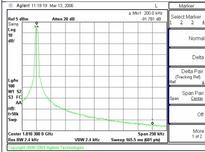
Spur at 200 kHz offset at a worst case frequency of 1810.2 MHz is -91.7 dBc.
