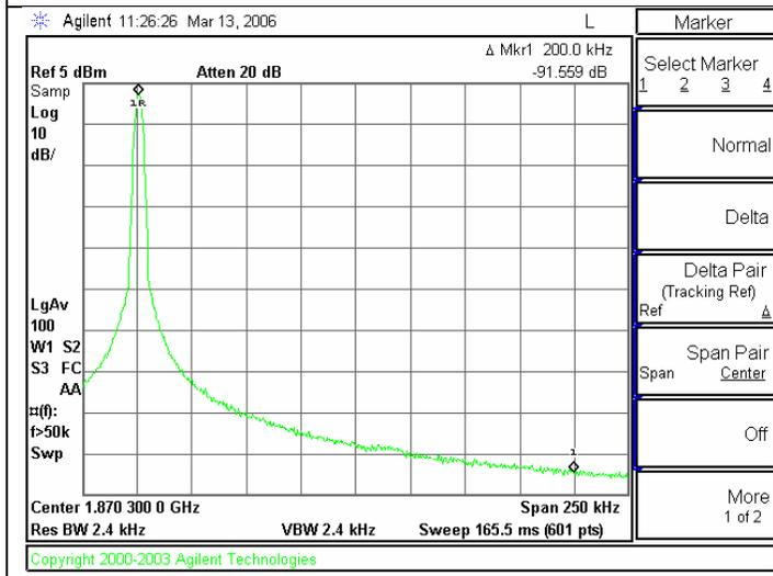
Spur at 200 kHz offset at a worst case frequency of 1870.2 MHz is -91.5 dBc.
