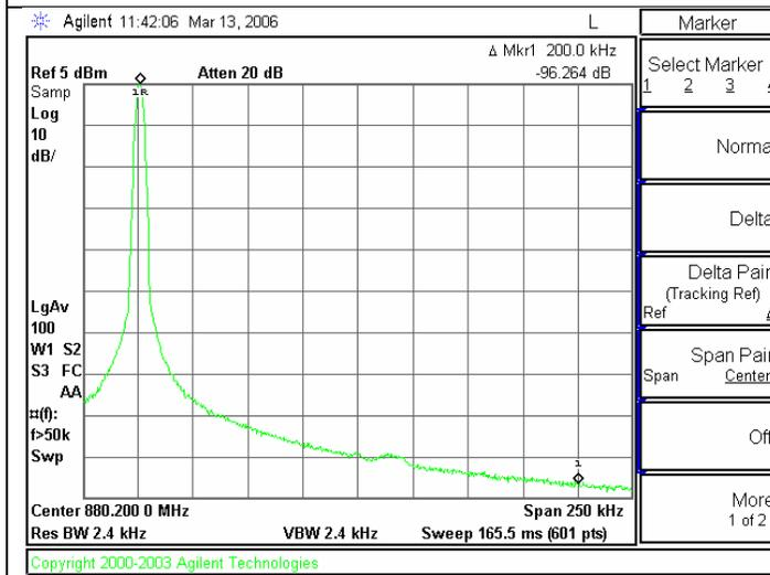
Spur at 200 kHz offset at a frequency of 880.1 MHz is -96.2 dBc. Since this mode uses the divide by 2 mode, the channel spacing here is actually 100 kHz. The spur at 100 kHz could be eliminated by doubling the channel spacing before the divider. The reason that the spur at 200 kHz is shown is to illustrate the theoretical 6 dB impact of the divider.
