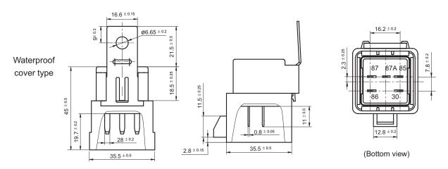
Notes: Terminal vertical deviation tolerance is 0.2mm.
