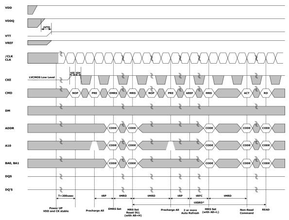
\* 200 cycle(tXSRD) of CK are required (for DLL locking) before Read Command
