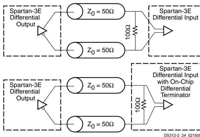
Figure 8: Differential Inputs and Outputs
