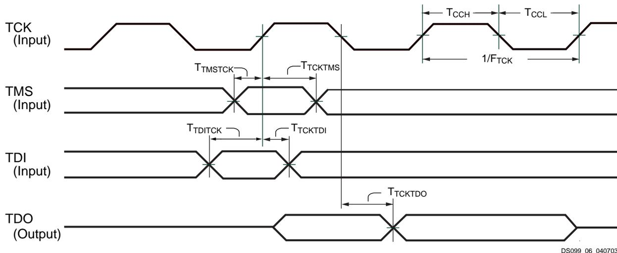
Figure 6: JTAG Waveforms
