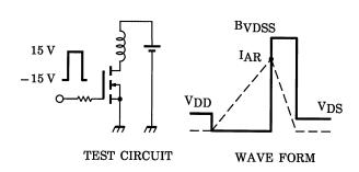
$$\begin{aligned} &RG = 25~\Omega \\ &V_{DD} = 90~V,~L = 6.36~mH \end{aligned} \qquad E_{AS} = \frac{1}{2} \cdot L \cdot I^2 \cdot \left( \frac{B_{VDSS}}{B_{VDSS} - V_{DD}} \right) \end{aligned}$$
