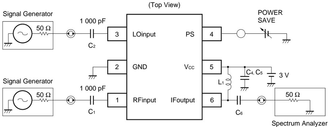
ILLUSTRATION OF THE TEST CIRCUIT ASSEMBLED ON EVALUATION BOARD
