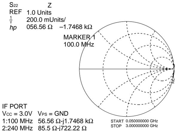
★ S-PARAMETERS OF IF OUTPUT MATCHING ( $V_{CC} = V_{PS} = V_{IFout} = 3.0\text{ V}$ ) –ON TEST CIRCUIT–
