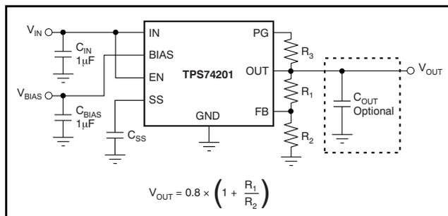
**Figure 26. Typical Application Circuit for the TPS74201 (Adjustable)**
