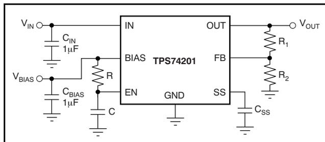
**Figure 29. Soft-Start Delay Using an RC Circuit on Enable**
