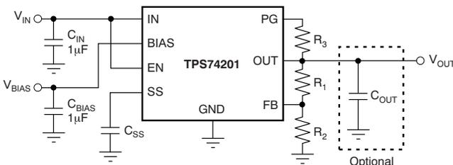
**Figure 1. Typical Application Circuit for the TPS74201 (Adjustable)**
