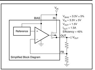
Figure 28. Typical Application of the TPS74201 Without an Auxiliary Bias
