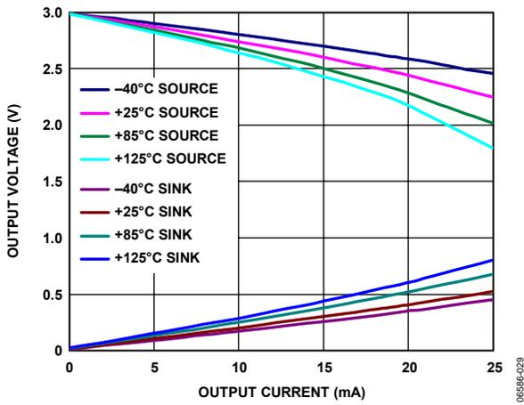
Figure 28. Output voltage Swing vs. Output Current, V<sub>S</sub> = 3 V
