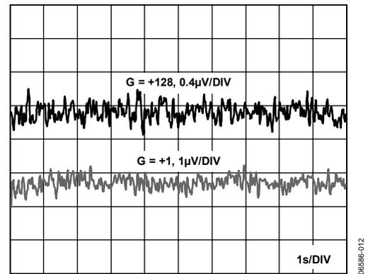
Figure 8. 0.1 Hz to 10 Hz Noise
