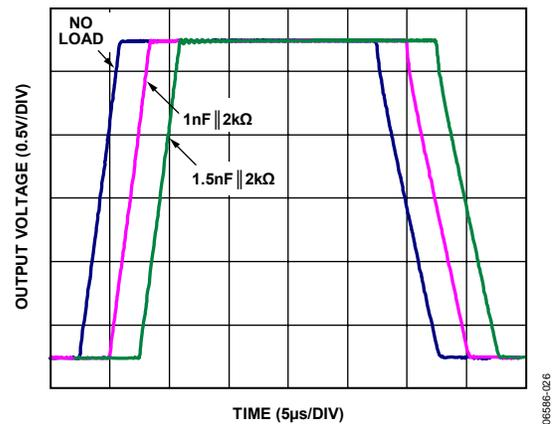
Figure 26. Large Signal Transient Response,  $V_S = 3\text{ V}$
