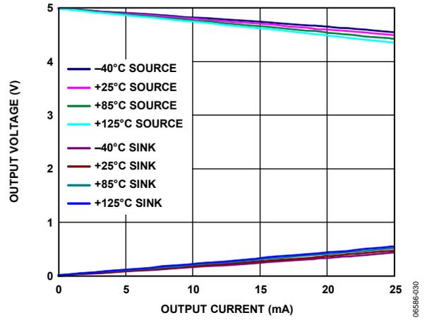
Figure 29. Output Voltage Swing vs. Output Current, V<sub>S</sub> = 5 V
