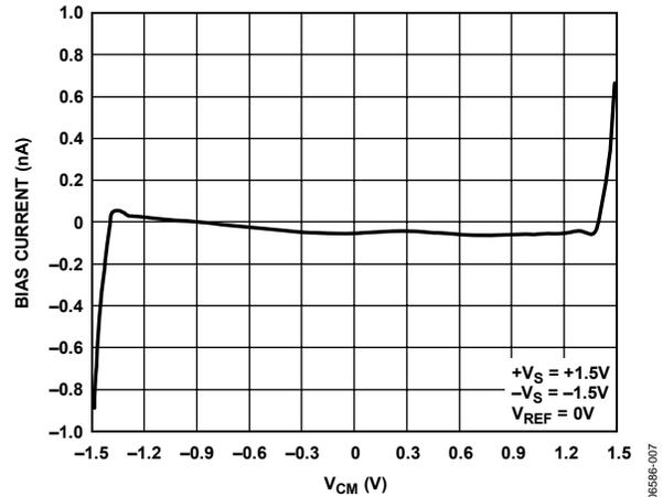
Figure 12. Bias Current vs. Common-Mode Voltage, 3 V
