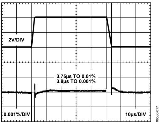
Figure 17. Large Signal Pulse Response,  $G = 8$ ,  $V_S = 5\text{ V}$
