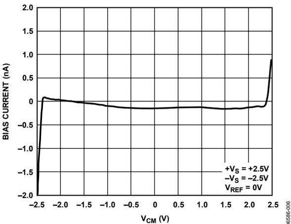
Figure 11. Bias Current vs. Common-Mode Voltage, 5 V
