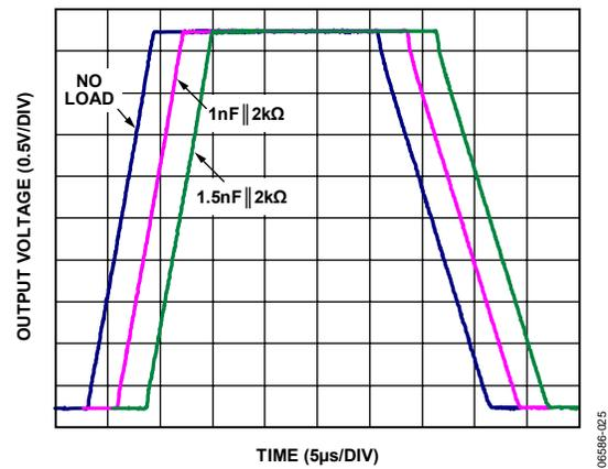
Figure 25. Large Signal Transient Response,  $V_S = 5\text{ V}$
