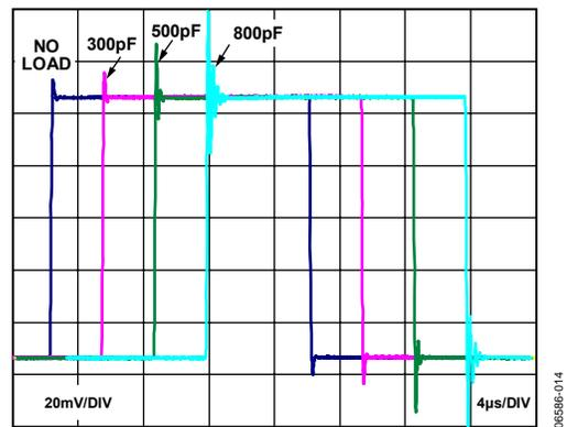
Figure 14. Small Signal Pulse Response for Various Capacitive Loads,  $G = 1$
