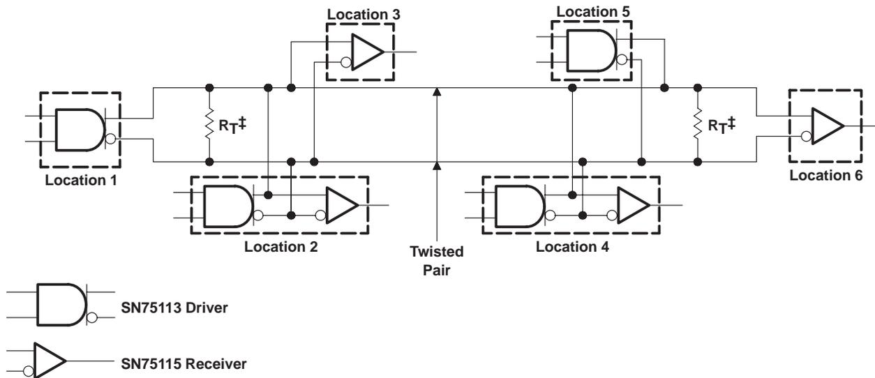
‡  $R_T = Z_O$ . A capacitor may be connected in series with  $R_T$  to reduce power dissipation.
