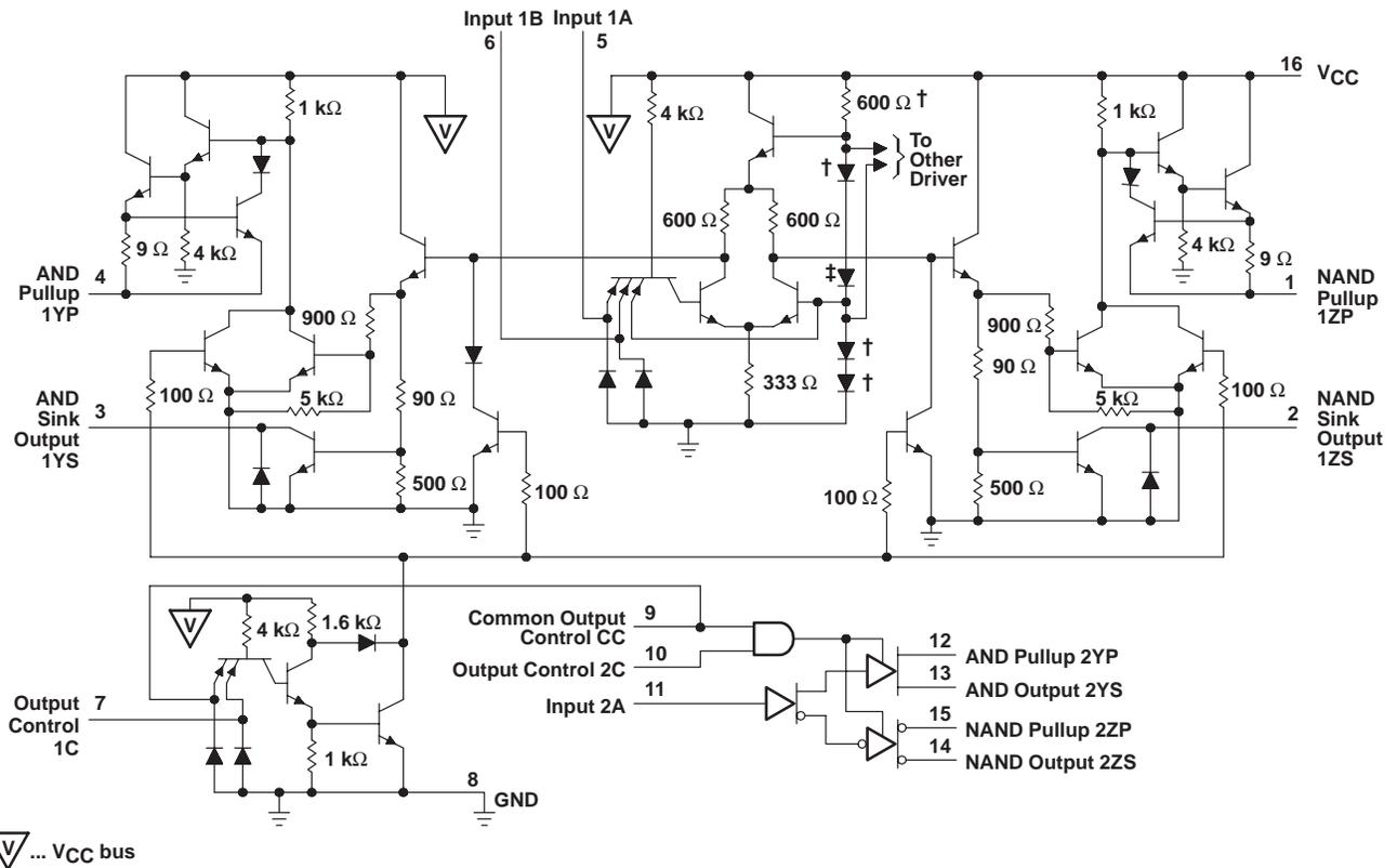
† These components are common to both drivers. Resistor values shown are nominal and in ohms.
