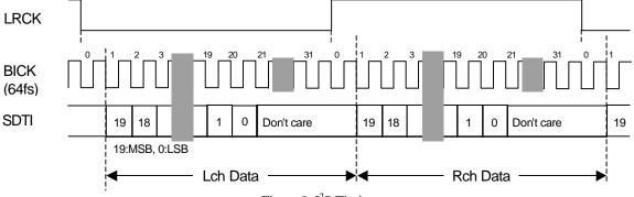
Figure 9. I<sup>2</sup>S Timing
