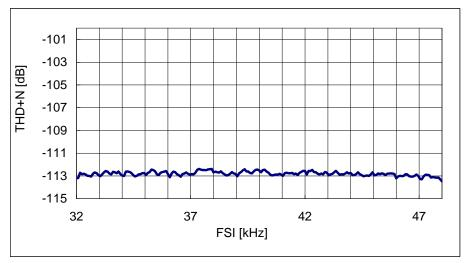
Figure 1: Input Sample Rate (FSI) vs. THD+N (FSO=48kHz)
