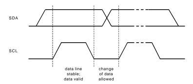
Figure 19. Bit transfer on the I<sup>2</sup>C-bus
