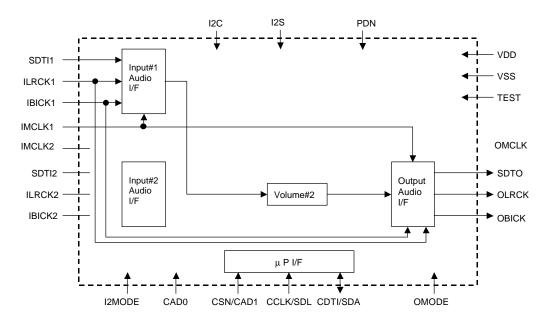
Figure 5. Path Mode 2 (Input#1 through output)
