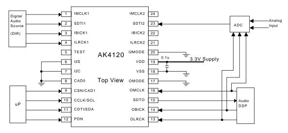
Figure 21. Example of a typical design
