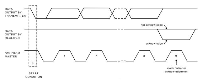
Figure 18. Acknowledge on the I<sup>2</sup>C-bus
