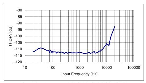
Figure 2: Input Frequency vs. THD+N (FSI=44.1kHz, FSO=48kHz)
