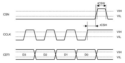
WRITE Data Input Timing (3-wire Serial mode)
