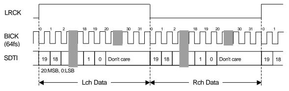
Figure 8. MSB justified Timing
