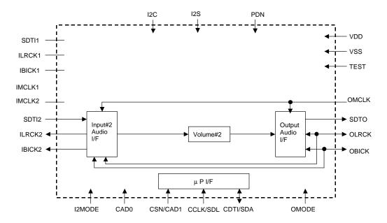
Figure 6. Path Mode 3 (Input#2 through output)
