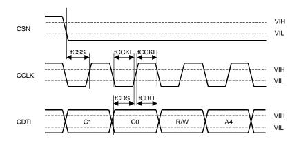
WRITE Command Input Timing (3-wire Serial mode)
