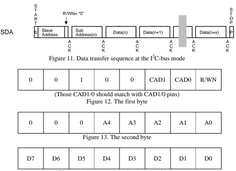
Figure 14. Byte structure after the second byte
