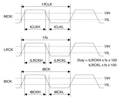
Figure 12. Clock Timing (EXT Slave mode)
