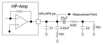
Figure 2. Headphone-Amp output circuit
