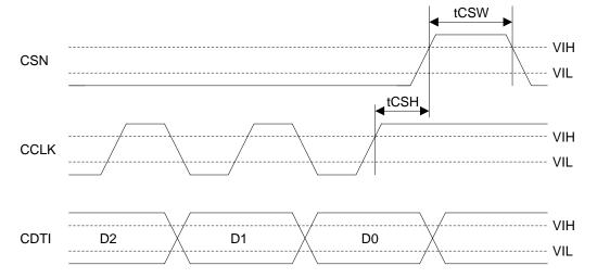
Figure 15. WRITE Data Input Timing
