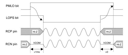
Figure 49. Power-up/Power-down Timing for Receiver-Amp
