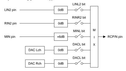
Figure 50. Receiver Mixing Circuit (AIN3 bit = "0", LOVL bit = "0")
