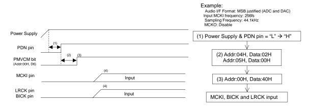
Figure 77. Clock Set Up Sequence (4)
