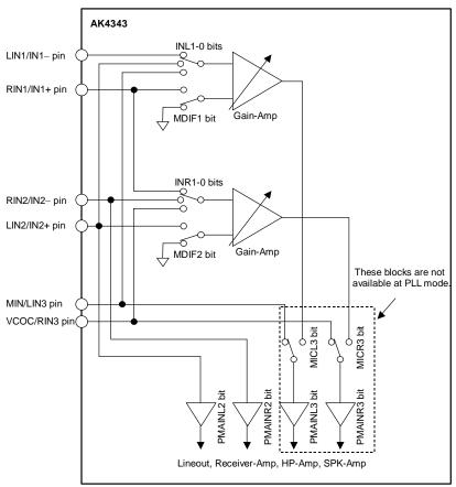
Figure 37. Analog Mixing Circuit
