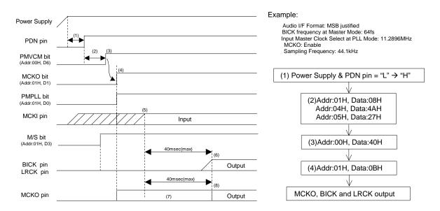
Figure 74. Clock Set Up Sequence (1)
