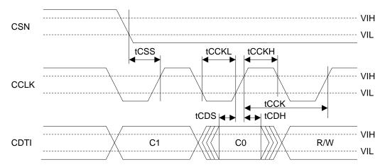
Figure 14. WRITE Command Input Timing
