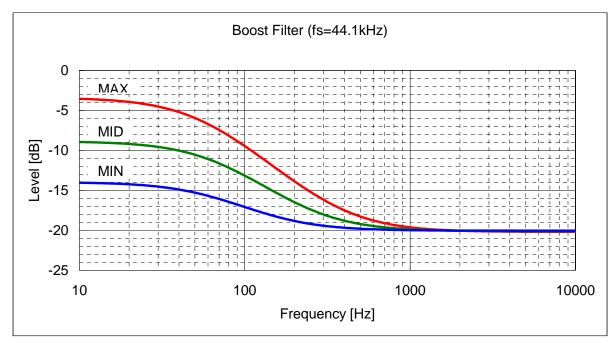
Figure 35. Bass Boost Frequency Response (fs=44.1kHz)
