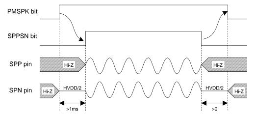
Figure 59. Power-up/Power-down Timing for Speaker-Amp
