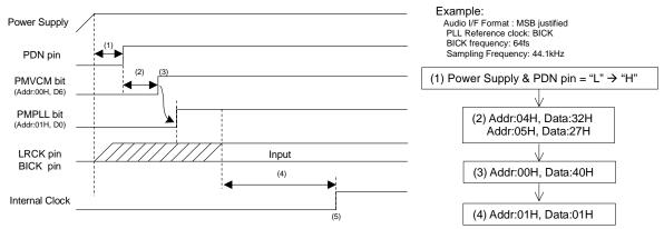
Figure 75. Clock Set Up Sequence (2)
