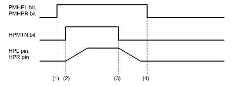
Figure 52. Power-up/Power-down Timing for Headphone-Amp
