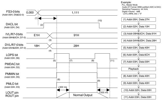
Figure 82. Stereo Lineout Sequence
