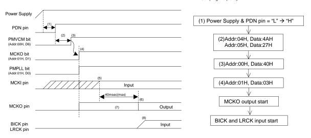
Figure 76. Clock Set Up Sequence (3)
