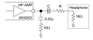
Figure 53. External Circuit Example of Headphone
