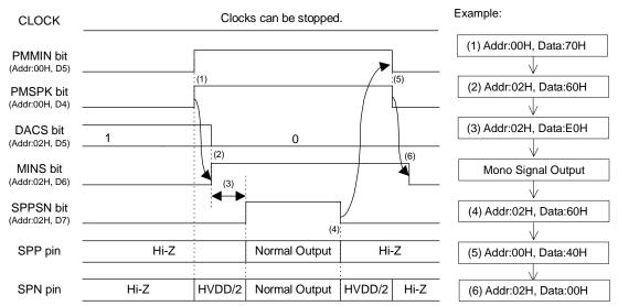
Figure 80. "MIN-Amp → Speaker-Amp" Output Sequence
