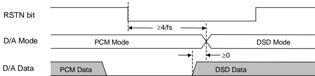
Figure 12. D/A Mode Switching Timing (PCM to DSD)
