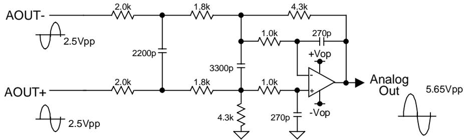
Figure 27. External 3rd order LPF Circuit Example
