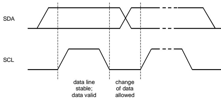
Figure 24. Bit transfer on the I<sup>2</sup>C-bus
