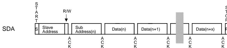
Figure 18. Data transfer sequence at the I<sup>2</sup>C-bus mode
