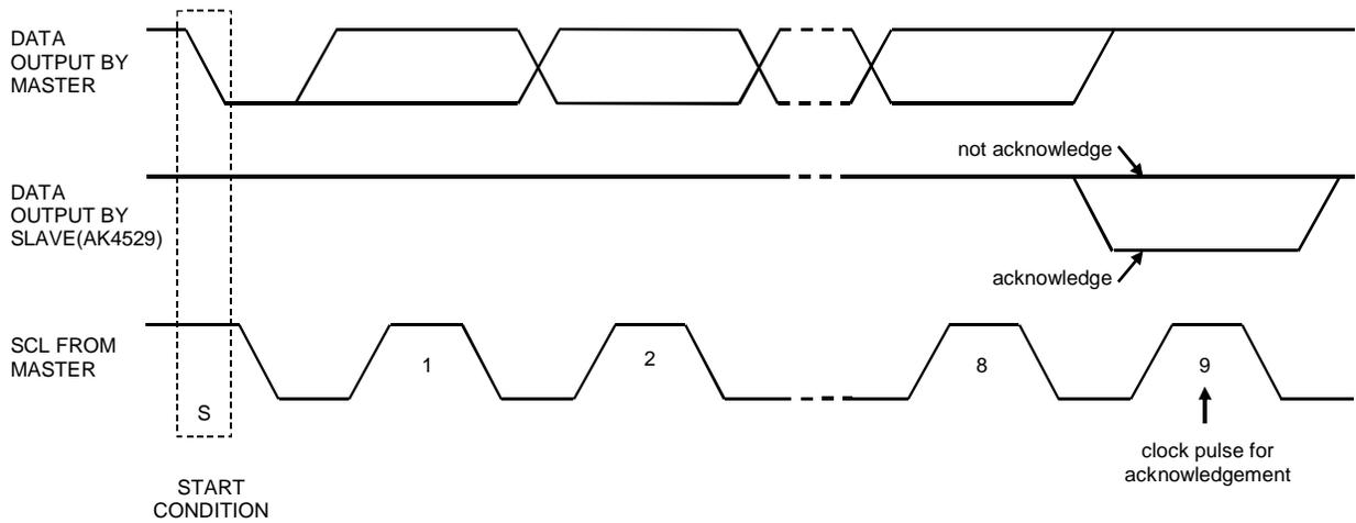
Figure 23. Acknowledge on the I<sup>2</sup>C-bus
