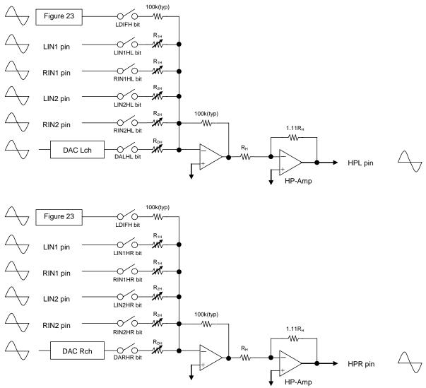
Figure 21. Summation circuit for HPL/R output
