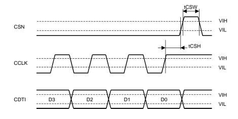
Figure 8. WRITE Data Input Timing
