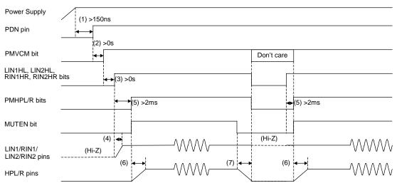
Figure 26. Power-up/down sequence of LIN1/RIN1/LIN2/RIN2 and HP-Amp
