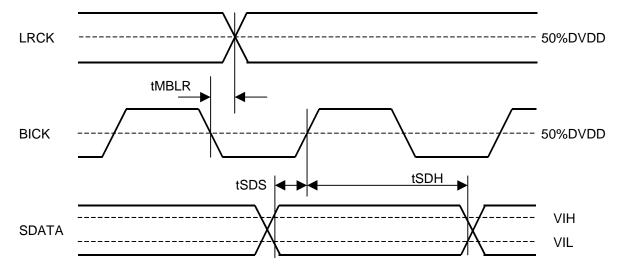
Figure 6. Serial Interface Timing (Master mode)
