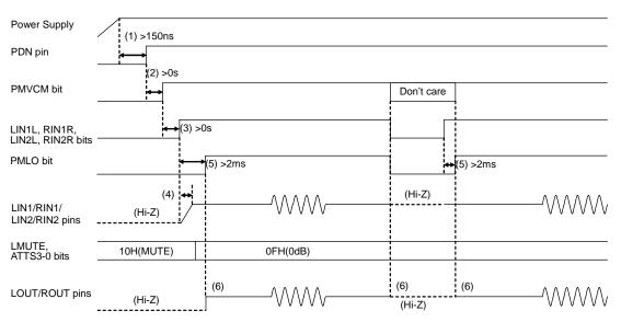
Figure 27. Power-up/down sequence of LIN1/RIN1/LIN2/RIN2 and Lineout
