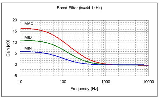
Figure 2. Boost Frequency (fs=44.1kHz)
