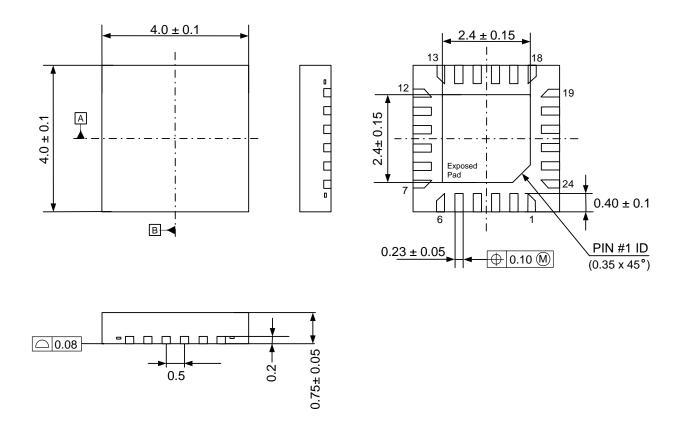
Note) The exposed pad on the bottom surface of the package must be open or connected to the ground.
