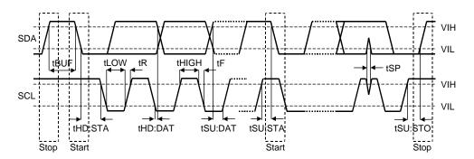
Figure 9. I<sup>2</sup>C Bus Mode Timing
