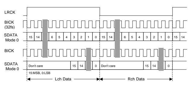
Figure 13. Mode 0 Timing (LRP = BCKP bits = "0")
