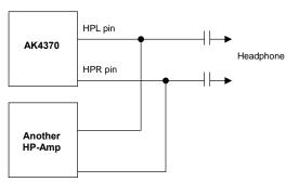
Figure 20. Wired OR with External HP-Amp
