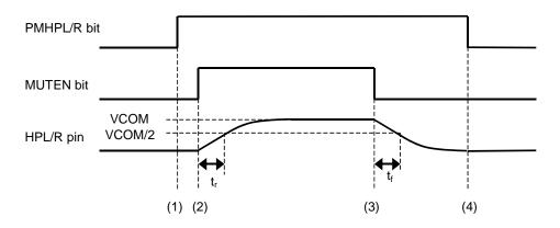
Figure 18. Power-up/Power-down Timing for the Headphone-Amp
