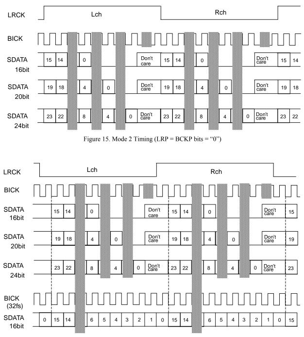
Figure 16. Mode 3 Timing (LRP = BCKP bits = "0")
