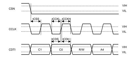
Figure 7. WRITE Command Input Timing
