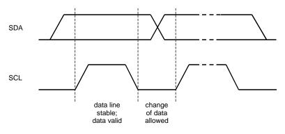
Figure 37. Bit Transfer on the I<sup>2</sup>C-Bus
