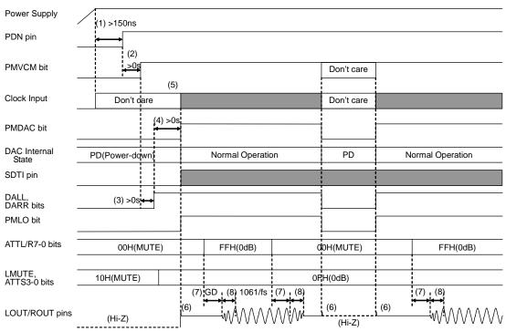
Figure 25. Power-up/down sequence of DAC and LOUT/ROUT (Don't care: except Hi-Z)
