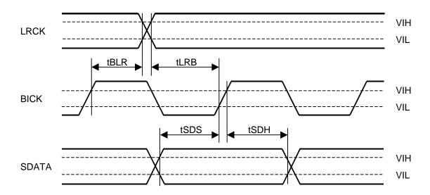
Figure 5. Serial Interface Timing (Slave Mode)
